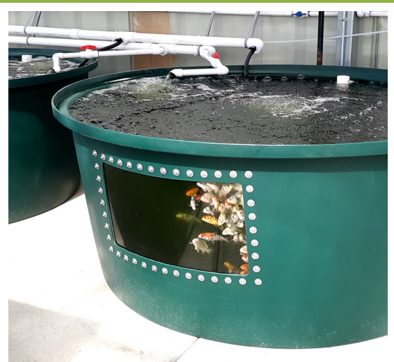
One of the four koi fish tanks at Bella Vita Farms. The nutrients produced by these fish are taken from the tank via pipes and distributed to the plants growing throughout the facility.
